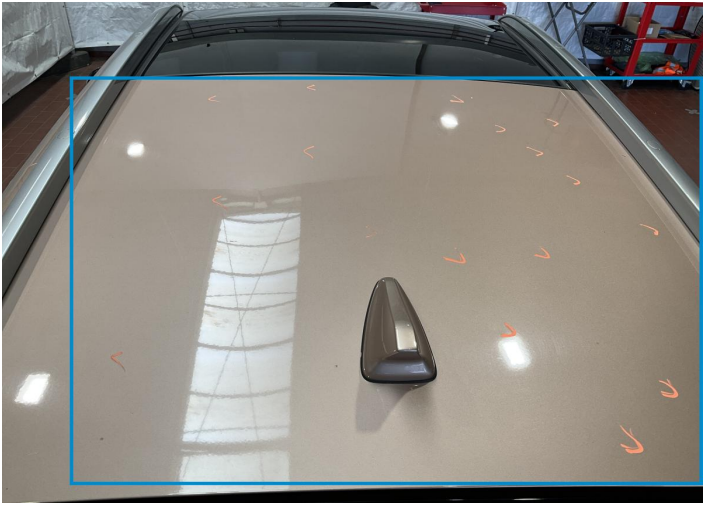
6. Roof Bodywork / Dent / Hail Area -
