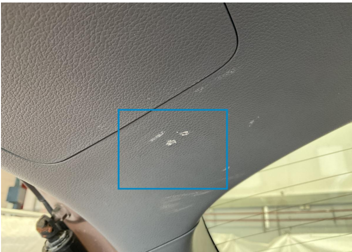
2. Tailgate Upholstery / Back Interior / Scraped -
