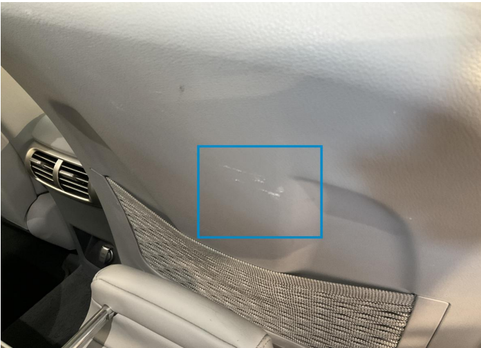
9. Backrest Cover / Front Right Interior / Scraped -
