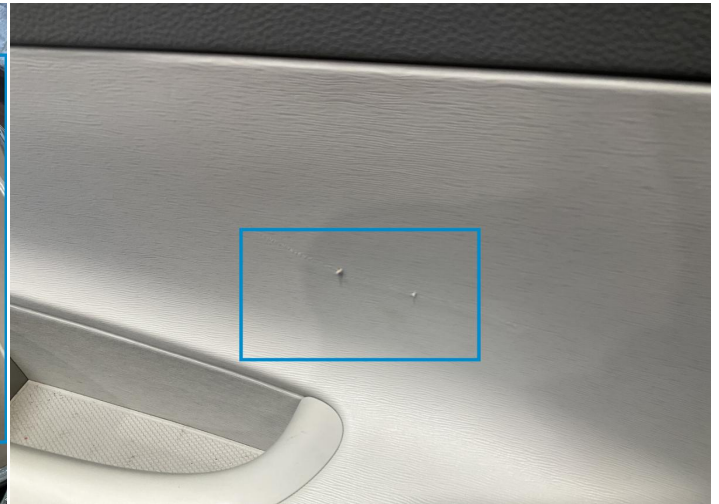
8. Panel Filling / Front Right Interior / Scraped -
