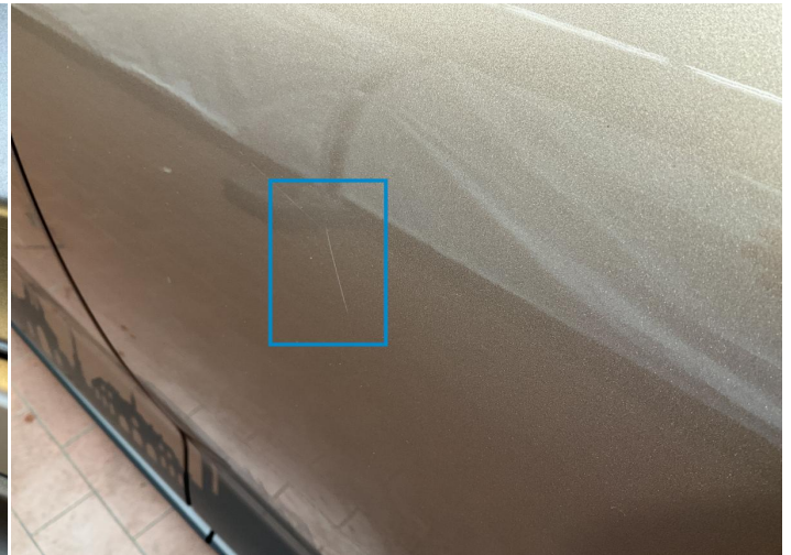
14. Door / Back Left Paint / Scratch / Scuff -
