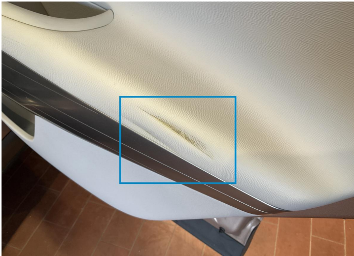
15. Interior door handle Back right Interior / Scraped -
