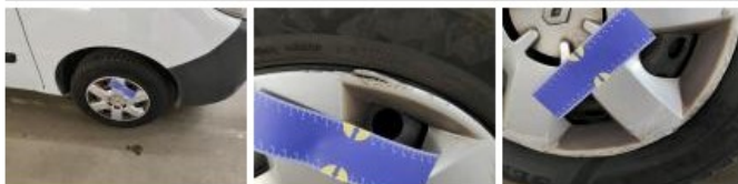
Wheel cover RR, Missing, Replace
