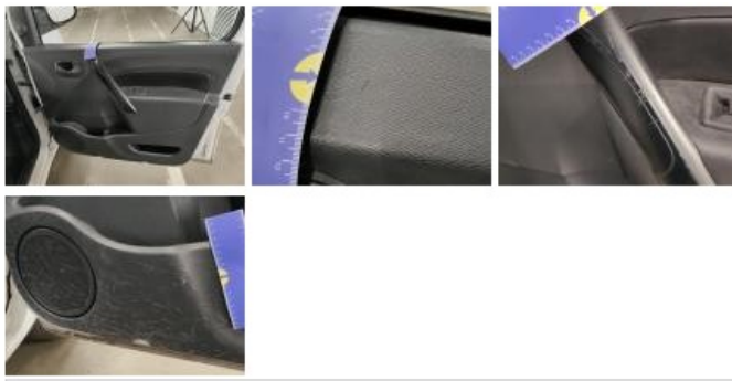
Centre console, Scratch(es), Smart repair
