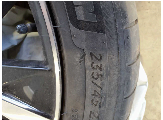
Damage 11: 2nd wheel set: 2 tyres - Does not meet the leasing specifications - Replace
