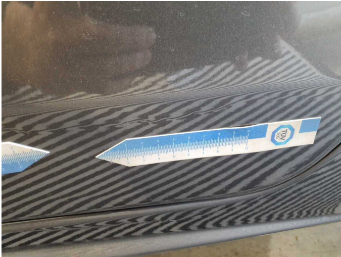
Damage 12: Door - rear left side: Door (Läufer) - Unprofessionally repaired - Repair and paint
