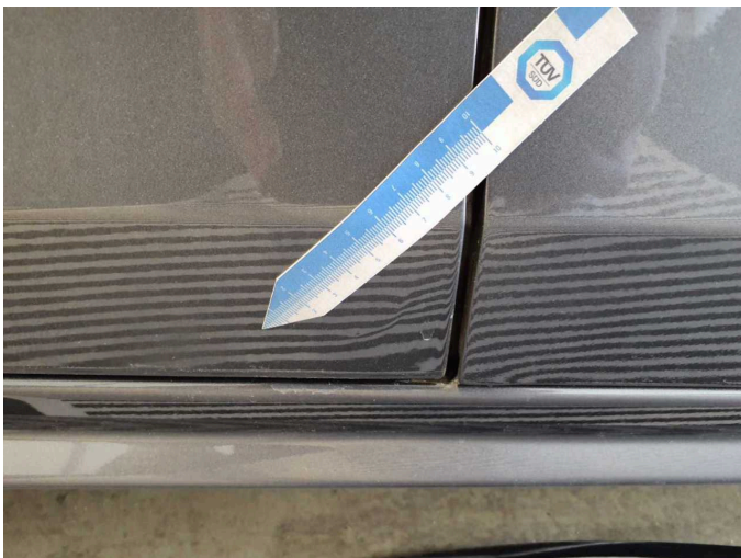
Damage 13: Door - front left side: Door - Deformed - Repair and paint
