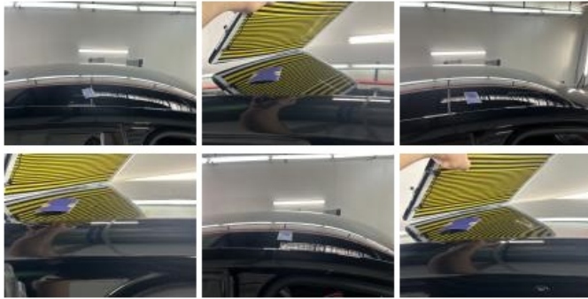
Roof, Dent(s), Paintless dent repair
