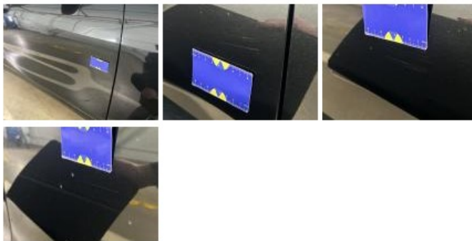
Door RR, Bad repair, Check
