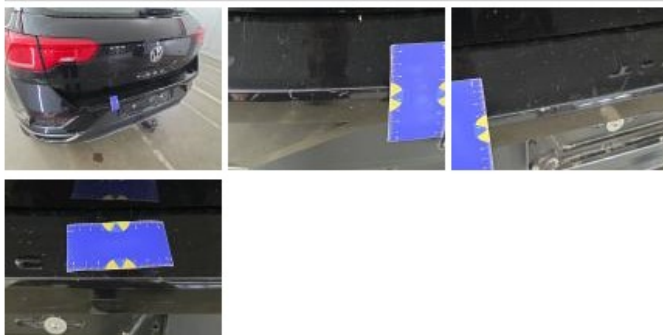
Step R, Dent(s), Paintless dent repair
