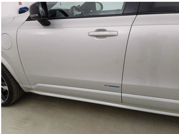
Beschädigung #4: Tür vorn links: Tür - Steinschlag - Smart Repair
