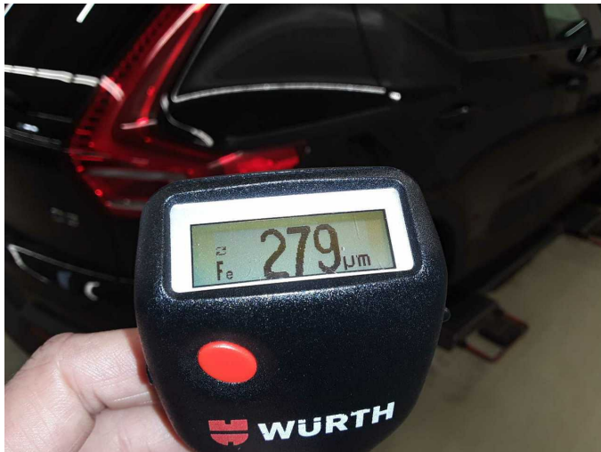
Side panel - rear right side: 279 µm
