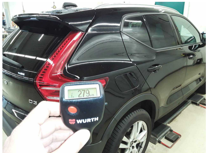
Side panel - rear right side: 279 µm
